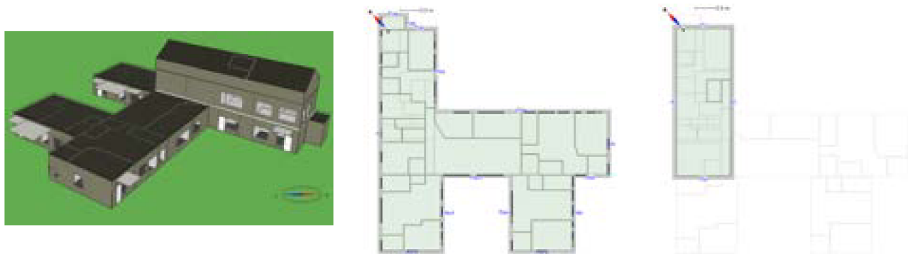
Figure 1: Model of the building in IDA-ICE (left), first floor plan (middle) and second floor plan (right).
