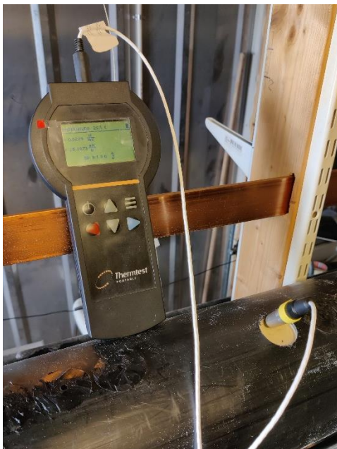
Figure 9: Measurement of thermal conductivity in a DH pipe
