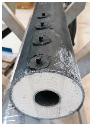
Figure 5: Restoration of a pipe after testing av adhesion strength
