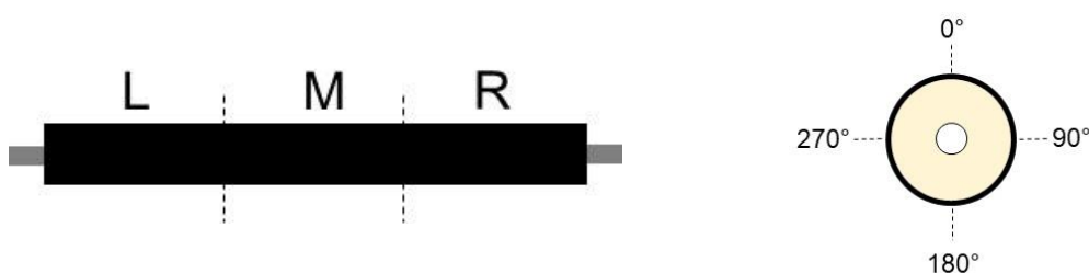
Figure 10: Sketch of where adhesion strength measurements have taken place
