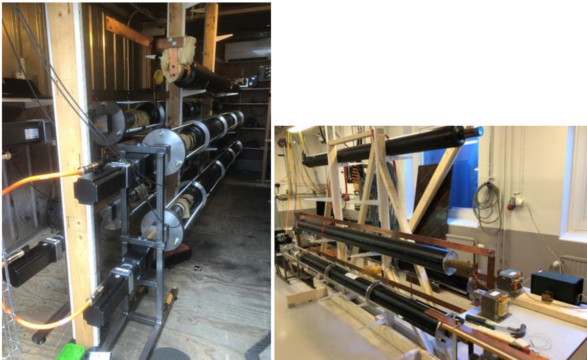
Figure 1: Pictures of set up for ageing of pipes using cycling load and temperature.
