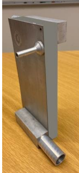
Figure 18: Prototype internal heat exchanger, design based on the experiences from the one shown in Figure 15.
