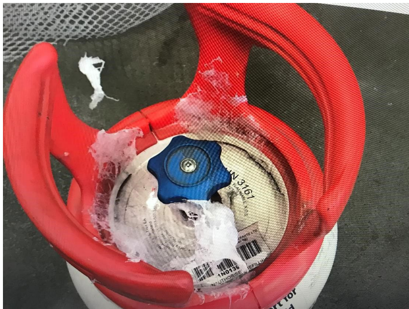
Figure 12: Bottle of R513A giving off a white foam when the valve is opened.
