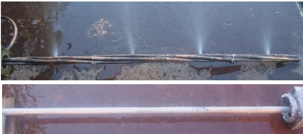
Figure 39. A Propac (top) and the Sanhua distributor (lower) evaluated with water-air mixture.
