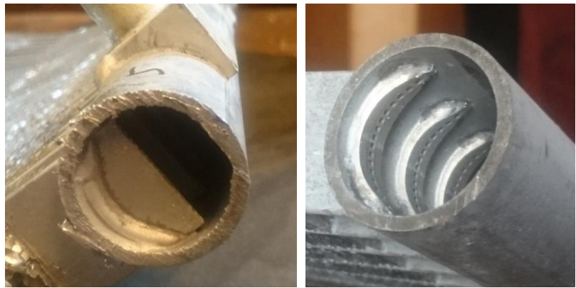
Figure 30. SD12 before and after sparking
